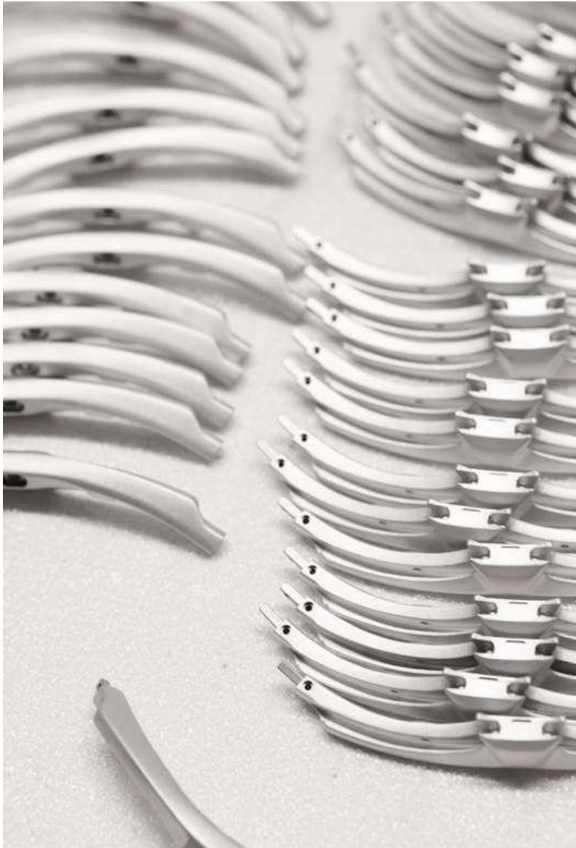
Fig. 2 MIM eyewear bridge sections after debinding, sintering and finishing at Matrix s.r.l.
