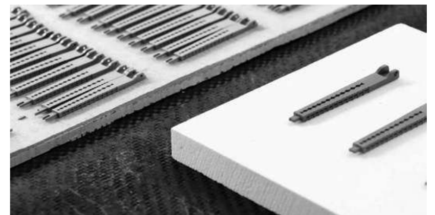
Fig. 4 The parts shown in Fig. 3 after debinding and sintering
