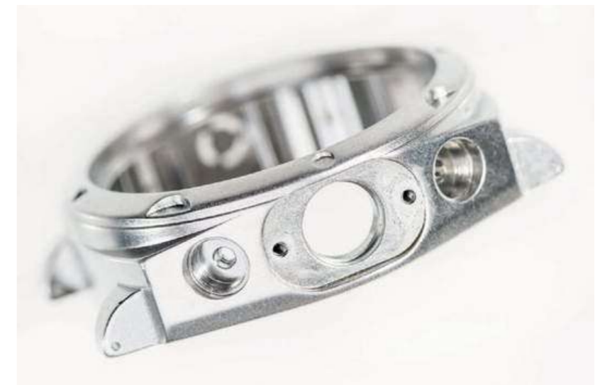
Fig. 8 A case for a diving watch. The original was made of bronze, but the change was made to MIM 316L for improved salt water corrosion resistance
