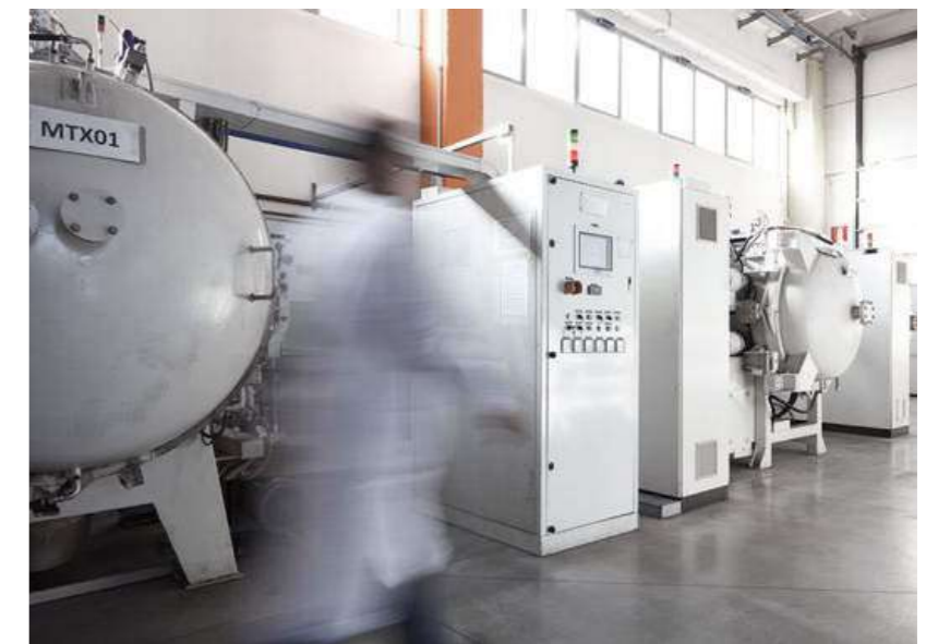
Fig. 1 Industrial-scale sintering furnaces for metal injection moulded part production at Matrix s.r.l.
