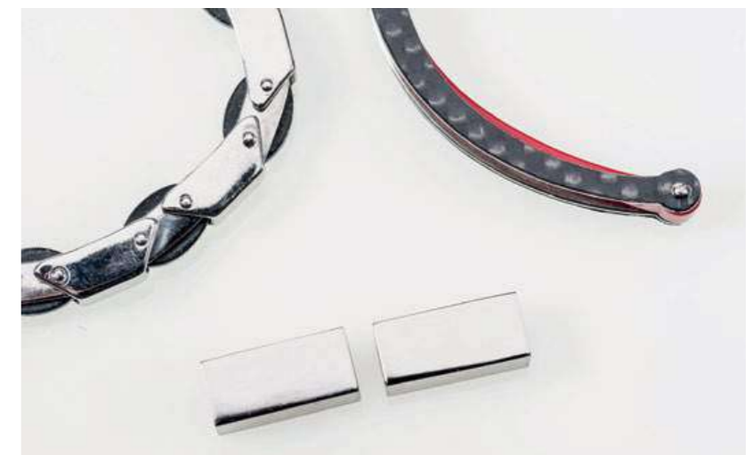
Fig. 9 Fashion bracelet components made by MIM
