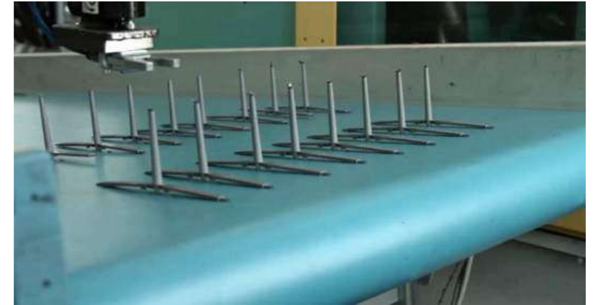
Fig. 3 MIM eyewear 'side arm' components as moulded and with the sprue still attached. The parts are removed from the mould by a robotic arm and, prior to debinding and sintering, the sprues are removed and re-ground for re-use
