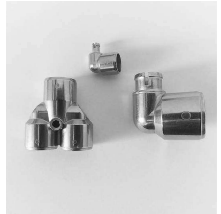
Fig. 11 MIM ventilator components produced by Matrix. The part diameters are 10, 15 and 20 mm
